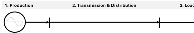
Figure 2 Conventional graph-based representation of the power system & simplified representation. Conventional graph-based representation, where nodes and edges represent buses and transmission lines, emphasizing pairwise physical connections emphasizing pairwise and independent relationships.
